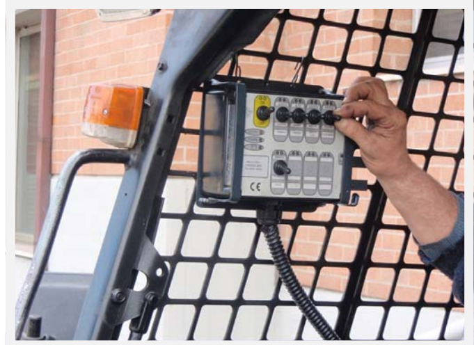
MG6 & MG7 Control Panel
