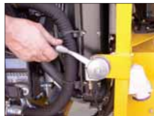
The Diesel engine speed is controlled by a handy lever.
