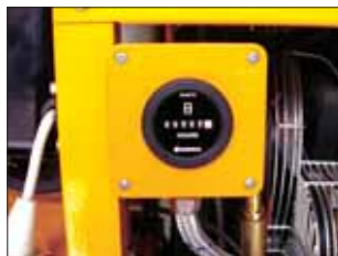
The hour-counter helps you to schedule work and maintenance.
